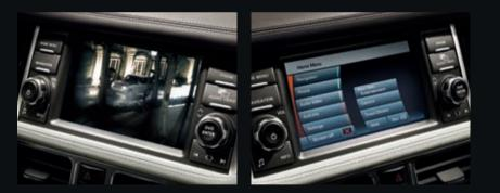
The Touch-screen with dual view technology uses 1,280 x 480 resolution, patented Parallax Barrier technology to display alternative columns of pixels to left and right-hand views, allowing driver and passenger to see different images.
